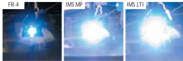
Light output of the same LED die on different circuit board materials at a maintained die temperature of 50°C.
